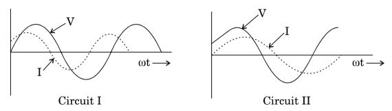
State, giving reason, in which of the circuits capacitive impedance  $(X_C)$  is (i) greater, (ii) smaller than the inductive impedance  $(X_I)$ .
